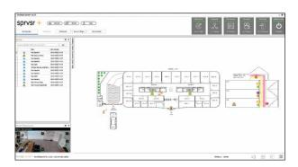
As in all systems, devices in the monitoring and control of card access systems are divided into two as input and output devices due to their duties. The list of devices in the system can be accessed via the "Card Pass" easy indicator in the upper right corner. The devices in the system can also be displayed on the map in the same way.
